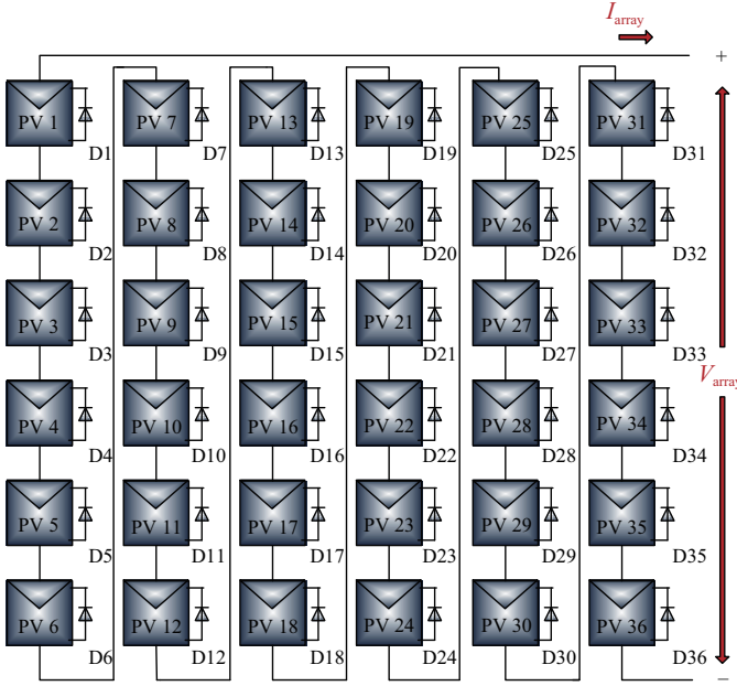
Fig. 5. MATLAB/Simulink model of 6 × 6 Series (S) PV array configuration.
