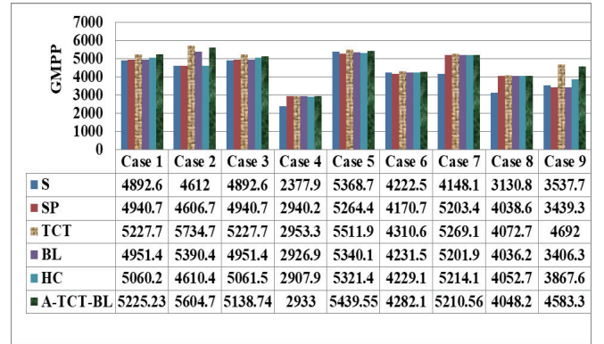
Fig. 18. GMPP of PV Configurations for different shading patterns.
